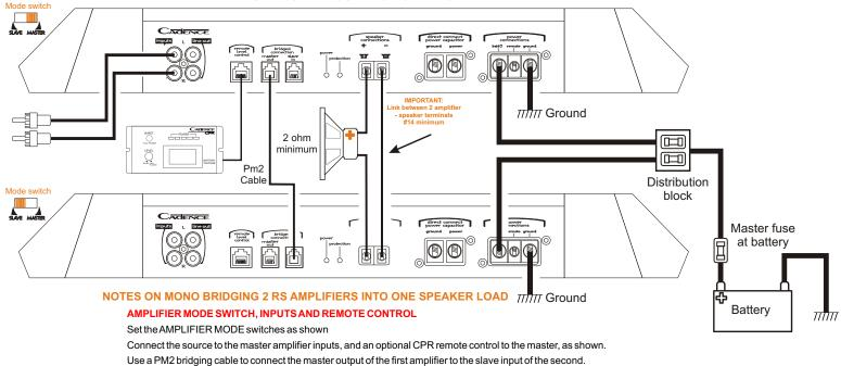
Connect the speaker as shown, with the link between the negative speaker terminals of the two amplifiers.
